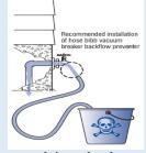
An ordinary garden hose submerged in a bucket of water or swimming pool can result in backflow
